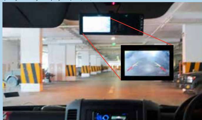
A Multi-role Utility Vehicle (MUV) Transporter installed with rear view cameras and distance guidelines to enhance the Transport Operator's (TO) view when reversing. Shown here is the display screen that the TO sees.
