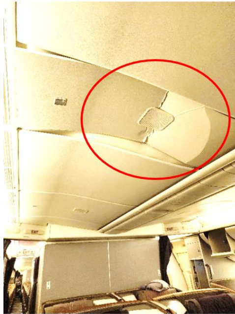
Figure 4: Broken ceiling panel
