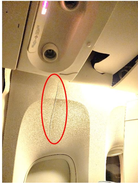
Figure 8: Cracked sidewall panel
