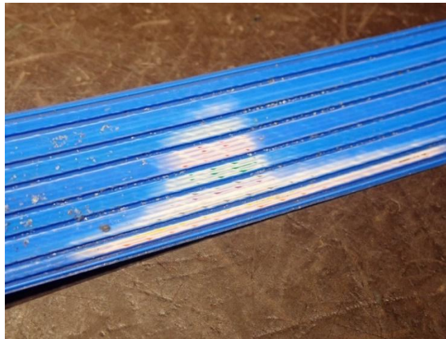
Figure 21: Conductor found exposed on Ribbon 1
