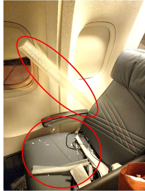
Figure 9: Broken sidewall light
