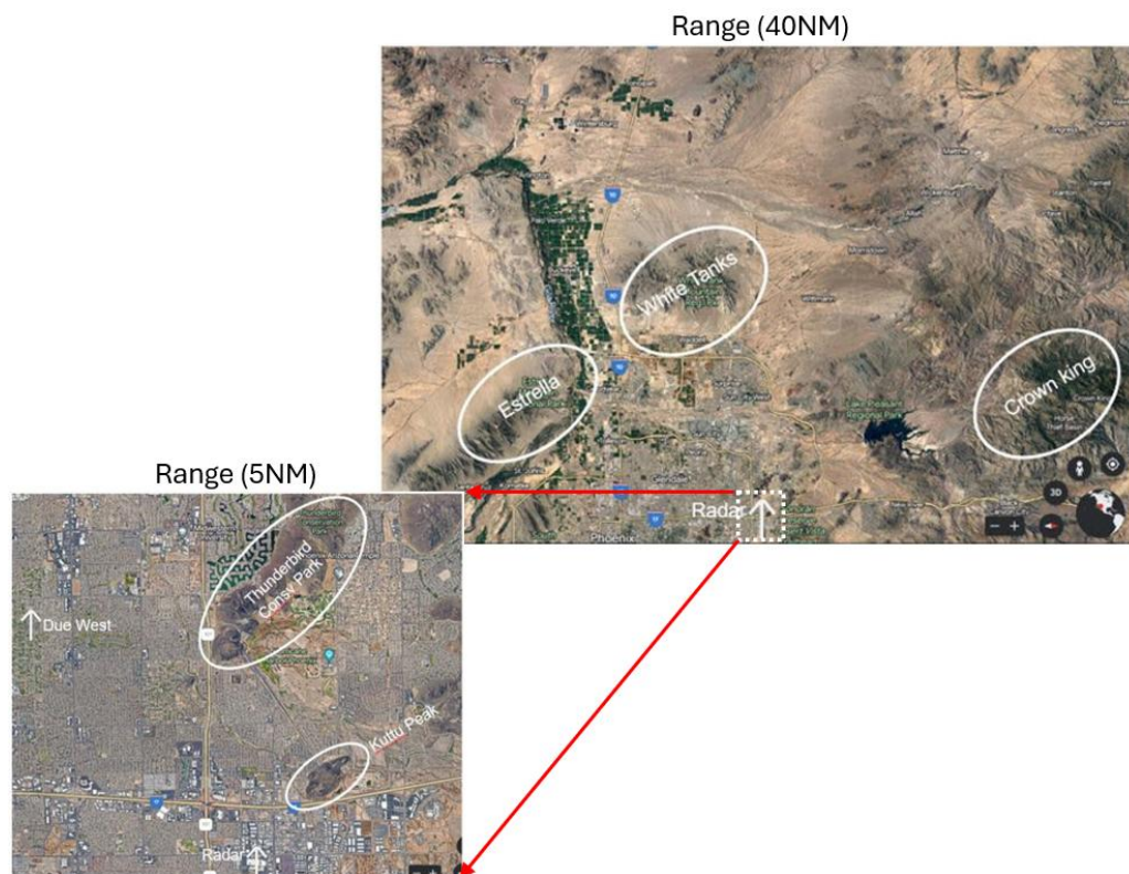
Figure 17: WXR transmission and reception operational test targets
