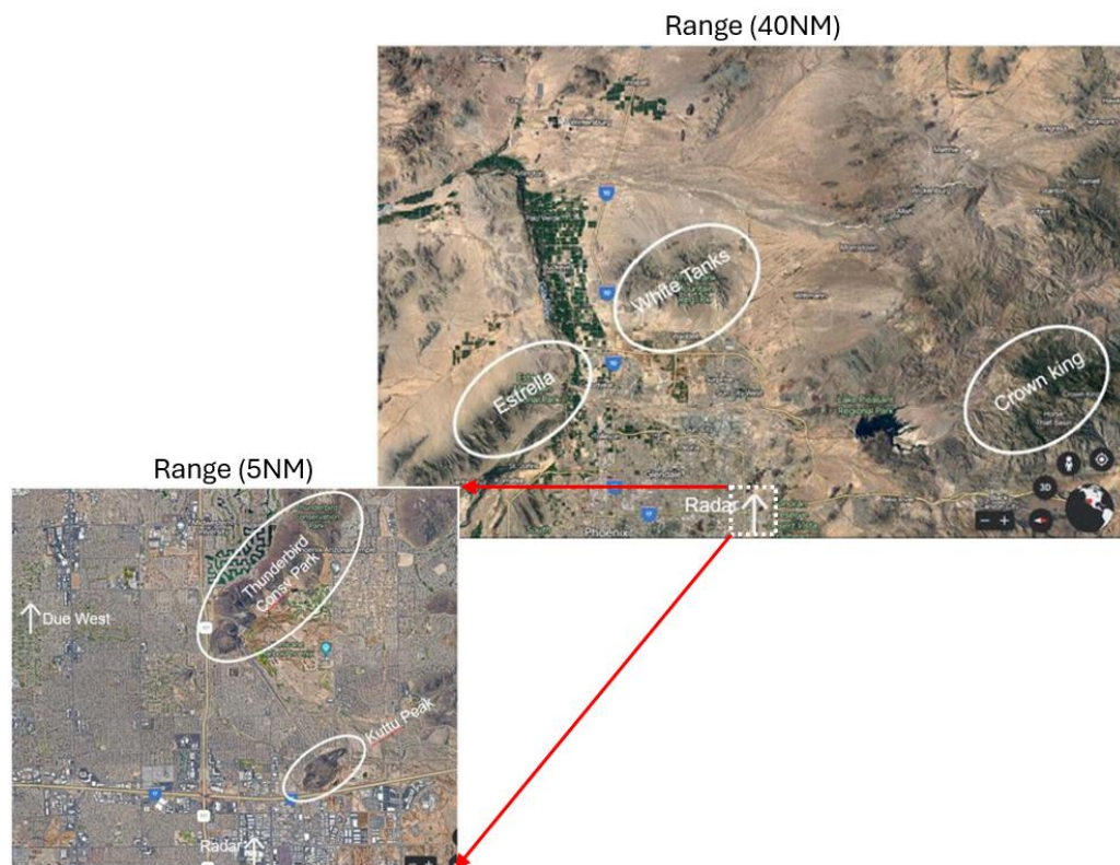
Figure 17: WXR transmission and reception operational test targets
