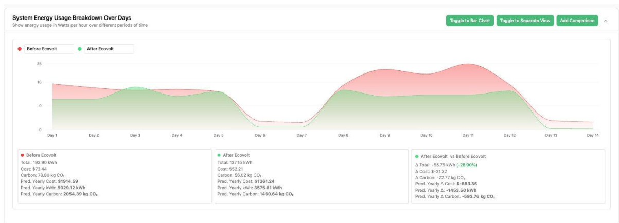
Figure 37. Overlaid daily comparison of the baseline (Before Ecovolt) and post-deployment (After Ecovolt) periods, with aggregate energy, cost, and carbon metrics. Charts generated by the Everest platform.
