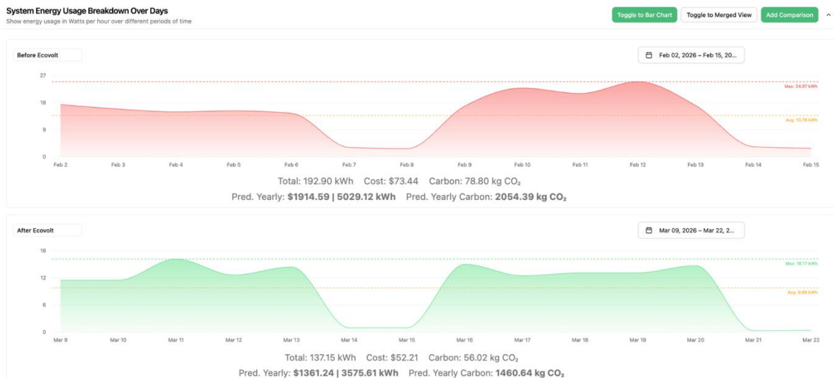
Figure 36. Daily plug-load consumption over the baseline fortnight (Before Ecovolt, upper) and the matched post-deployment fortnight (After Ecovolt, lower).
