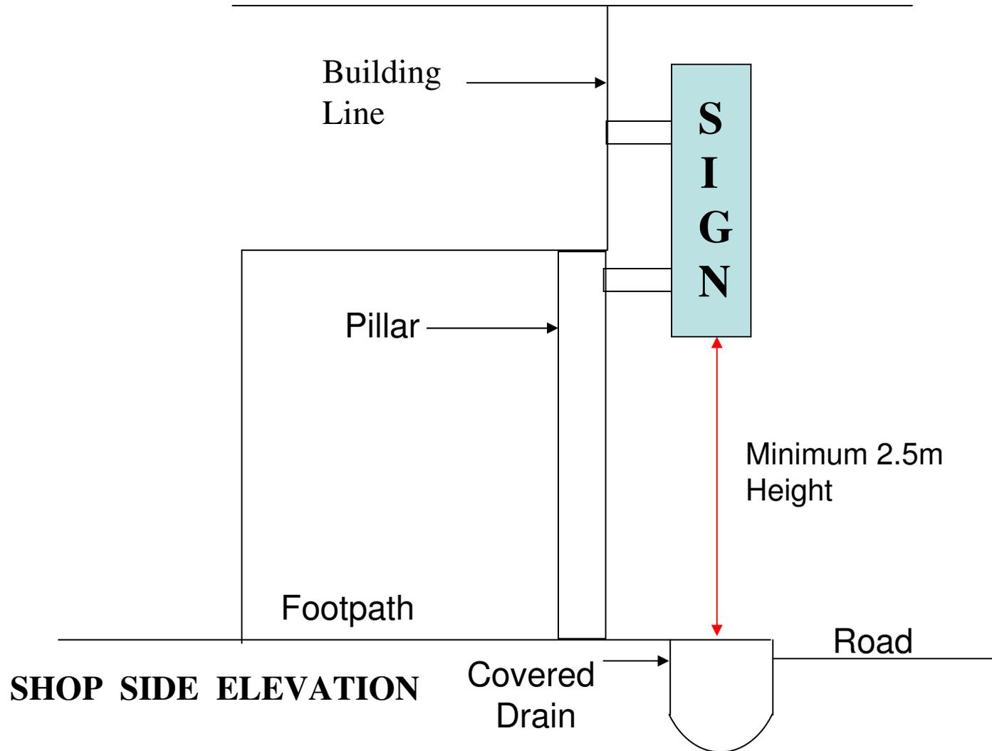
3. No advertisement, electronic billboard, signboard or skysign shall project over any street by more than 60 centimetres beyond the building line with a minimum height of 3.75 metres but less than 5 metres measured vertically from the roadway.
