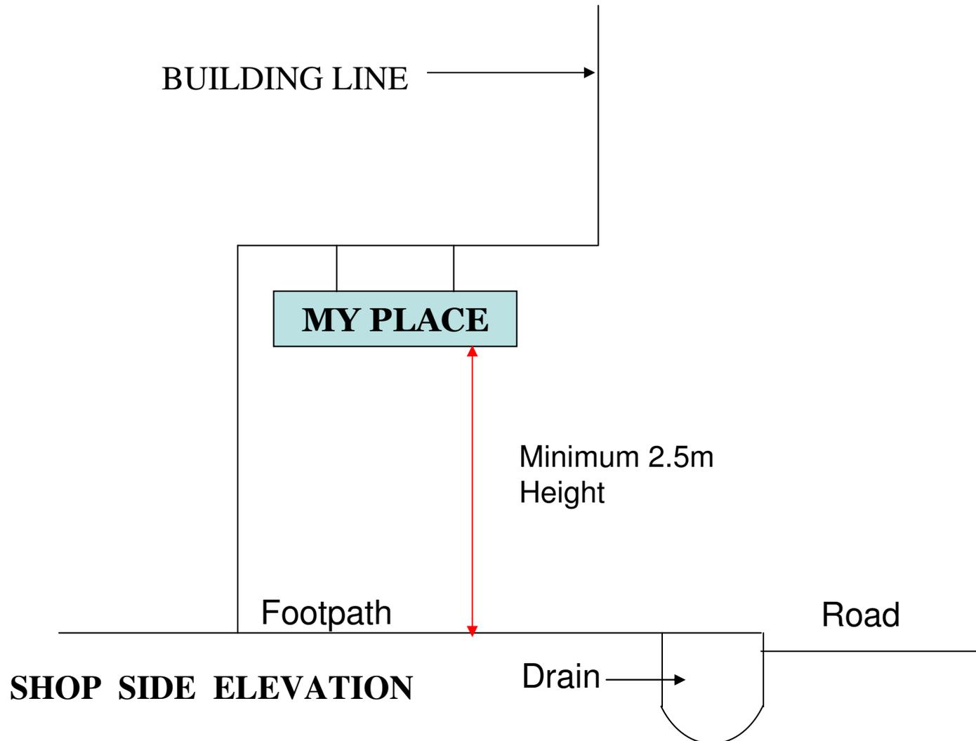
2. Where a roadside drain is covered, no advertisement, electronic billboard or signboard projecting over any street shall be erected less than 2.5 metres above the cover of the drain, measured vertically from the top of the cover to the underside of the advertisement, electronic billboard or signboard.
