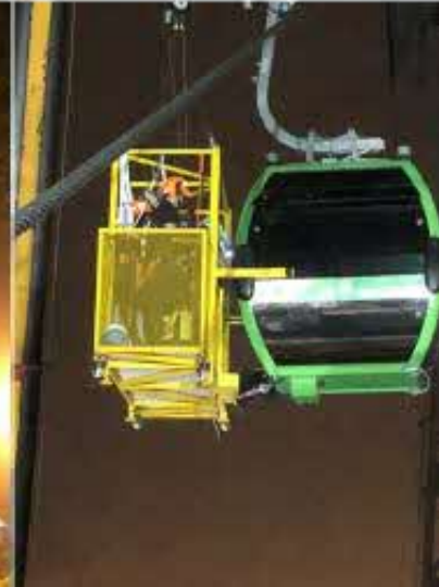
Rescue-Cage being anchored to the cabin
