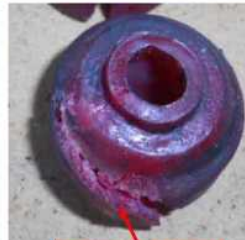
Damaged / Brittle PU Buffer
