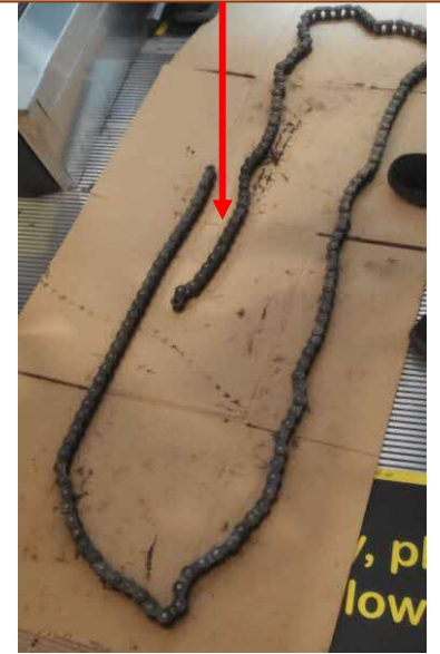
Broken Handrail Chain
