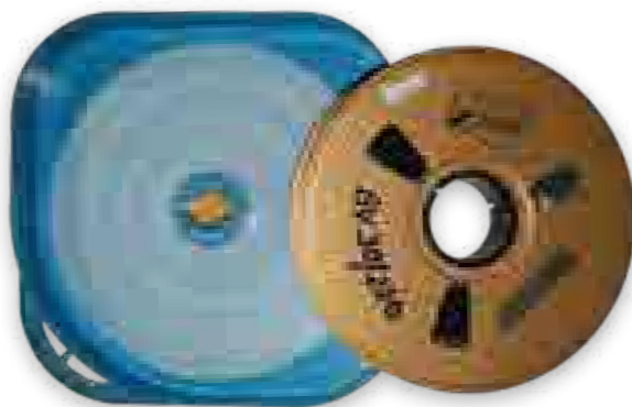
A two-inch quadruplex tape weighing 5.5 kg per tape. Courtesy of National Archives of Singapore.
