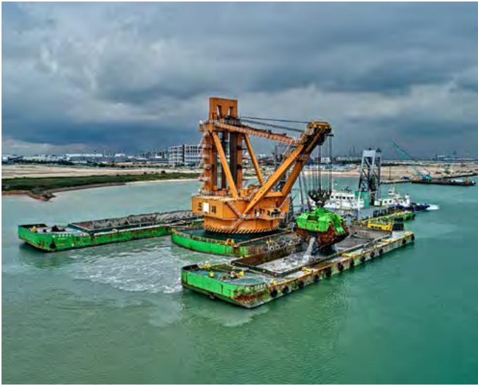
GOSHO—world's largest grab dredger currently deployed at Tuas for reclamation works
