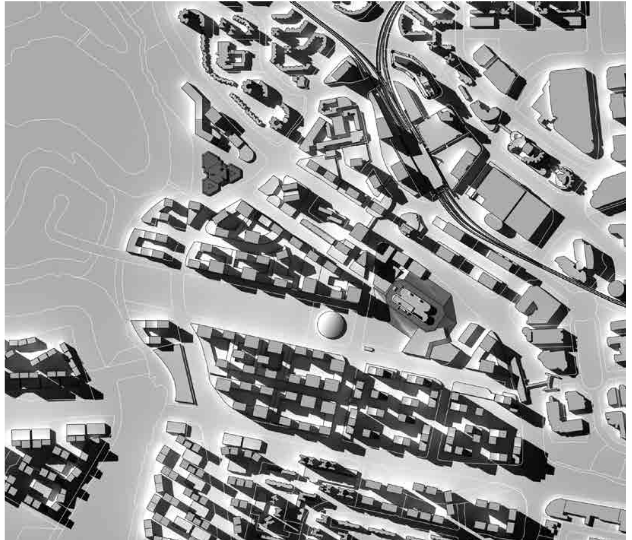
Shadow simulation of the precinct based on the sun's position on 21 June at 4pm
