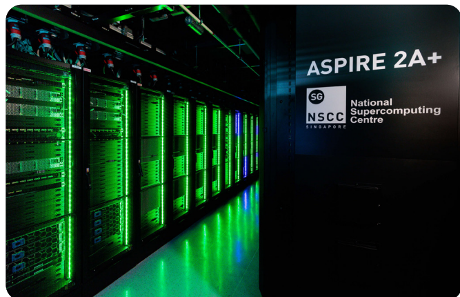
ASPIRE 2A+ – powered by 320 NVIDIA H100 GPUs, delivering 21.7 petaFLOPS based on theoretical peak performance.
