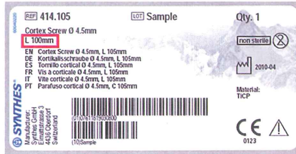
Figure 1 – Incorrect Label for Part 414.105
