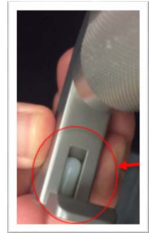
Figure 2: Image of melted slug
