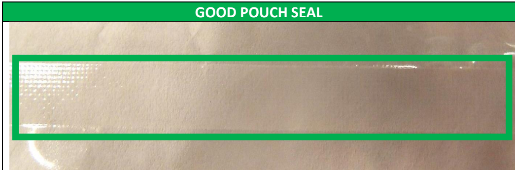
Figure 1 - Good Pouch Seal. Seal is not interrupted (close up view)
