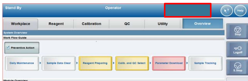
Figure 2: Date and time (in the red box) are not displayed in the Status Line of the User Interface
