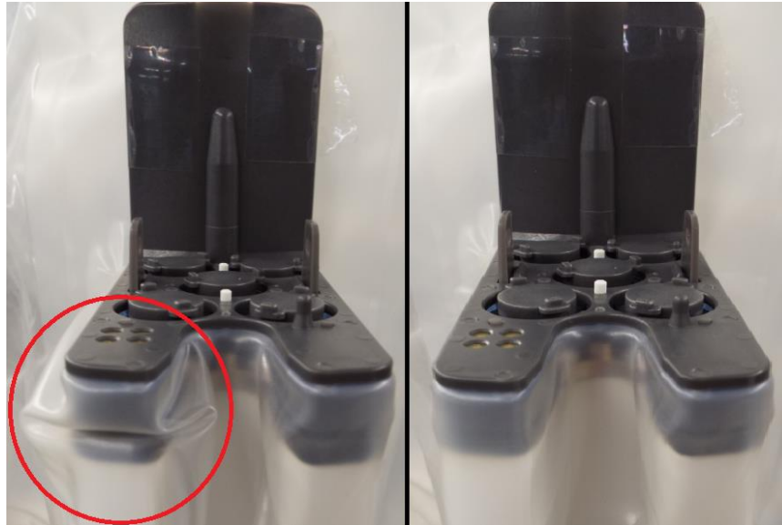
Figure 1. Pinched Drape Pouch (left) vs. Smooth Drape Pouch (right)
