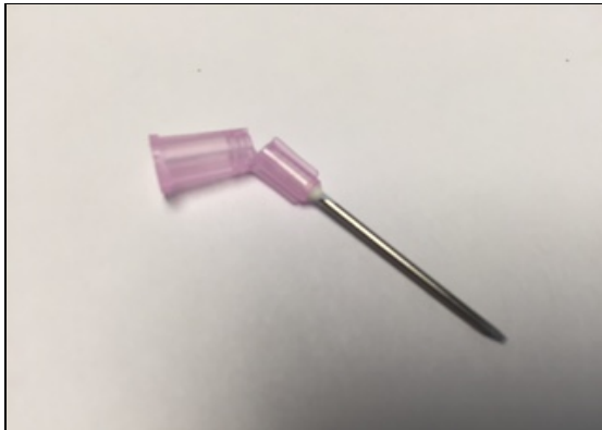
Figure 3- Cracked Hub (Worst Case)
