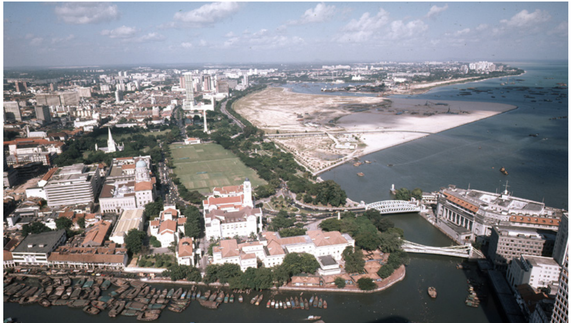
An overview in 1975 showing the first phase of land reclamation, known as Marina South and Marina Centre, to support the construction of the East Coast Parkway (ECP). Later land reclamation phases focused on the extension of the Central Business District.
