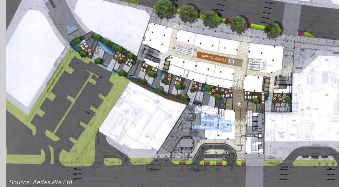
Staggering of ORAs along the pedestrian mall.
