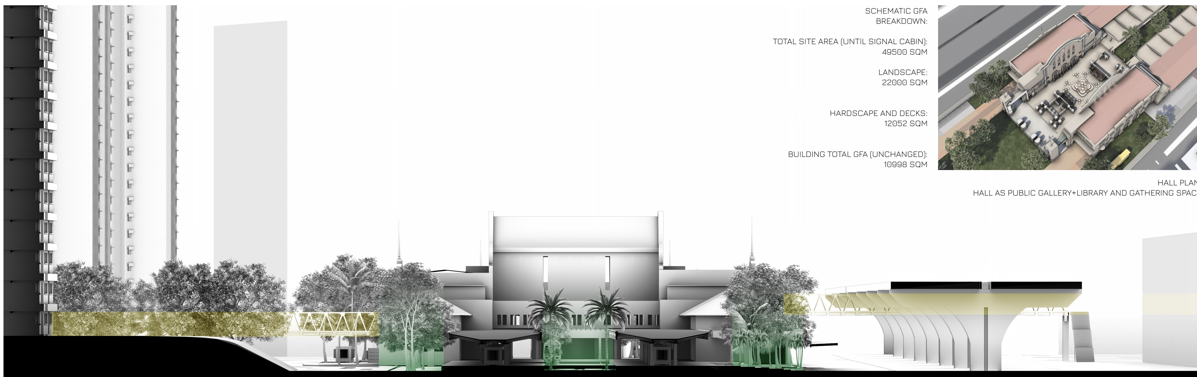
EXISTING HDB | EXISTING ELEVATED GROUND | NEW BRIDGE TO HDB AREA | LANDSCAPING + PEDESTRIAN | PLATFORM + CONTAINER SPACES | ENHANCED ELONGATED COURTYARD | PLATFORM + CONTAINER SPACES | NEW STREET ENTRANCE | KEPPEL ROAD + NEW BRIDGE TO CSW | KEPPEL VIADUCT | FUTURE GREAT SOUTHERN WATERFRONT
