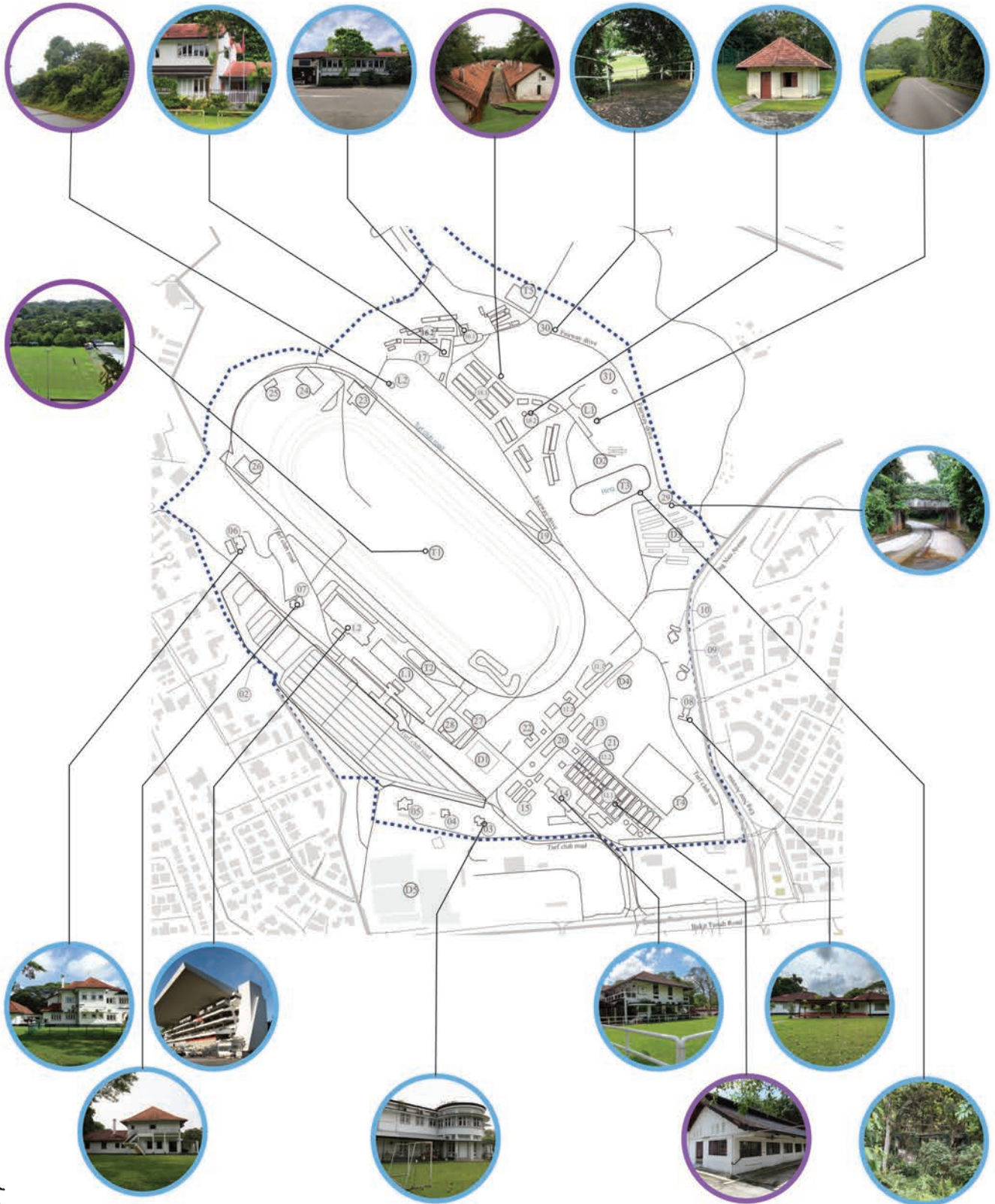
Figure 9.3: Diagram showing the buildings/ structure/ other elements scheduled for retention or partial retention/ demolition.
