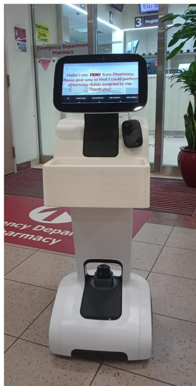
PillBot modified with a 3D printed storage box for medication delivery and transportation
