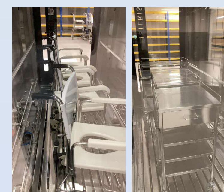
4 Load cleaned items to stainless steel cart and tow items to respective SGH block's tunnel
