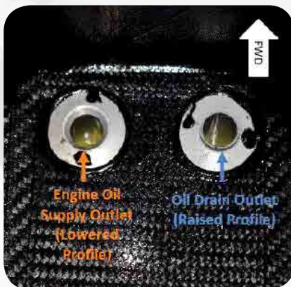
Figure 1: Incorrect Oil Tank Outlet Orientation (Top View)
