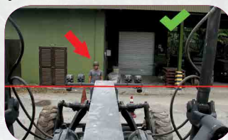
Figure 3. Front View of Operator from Motor Grader cabin: Incorrect (left) and Correct (right) Visual Cues
