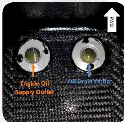
Figure 2: Correct Oil Tank Outlet Orientation (Top View)
