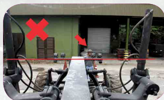
Figure 3. Front View of Operator from Motor Grader cabin: Incorrect (left) and Correct (right) Visual Cues
